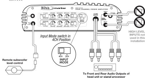
4-Channel Amplifier with 2-Channel Audio Input Source
