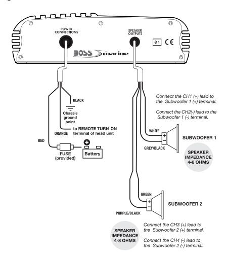
Tri-mode operation allows you to connect this amplifier to a pair of main speakers plus a subwoofer on one pair of output channels. The main speakers will operate in STEREO while the subwoofer simultaneously operates in MONO.
