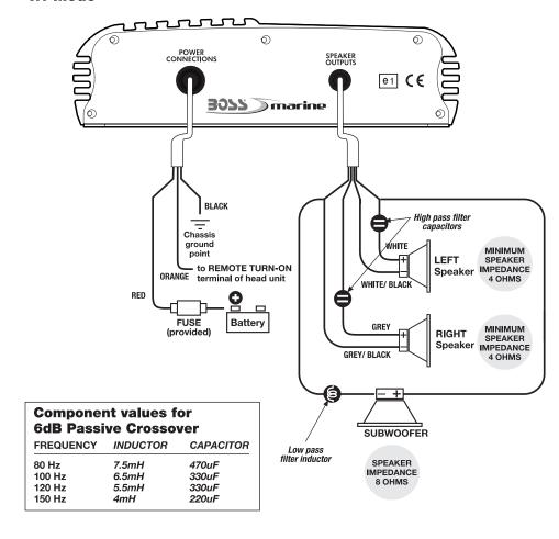
Tri-mode operation allows you to connect this amplifier to a pair of main speakers plus a subwoofer on one pair of output channels. The main speakers will operate in STEREO while the subwoofer simultaneously operates in MONO.
