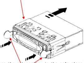
Note: Keep the <u>release key</u> in the safe place as you may need it in the future to remove the unit out
