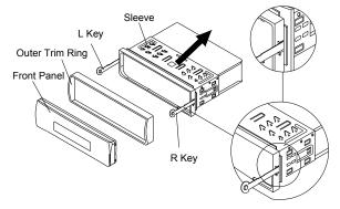
6. Mount the sleeve by inserting the sleeve into the opening of the dashboard and bend open the tabs located around the sleeve with a screwdriver. N will be able to make constant which ones will effective. Bending open the a tabs behind the dashboard the sleeve in place.
