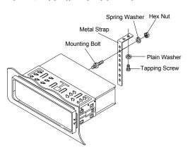
Reconnect the cable to the vehicle battery's negative (-) terminal. Then replace the outer trim ring and install the unit's front panel (see the steps of "installing the front panel").
